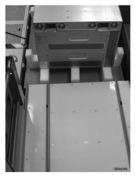
Figure 5. Lift tool positioned next to the chassis on the shipping tray
